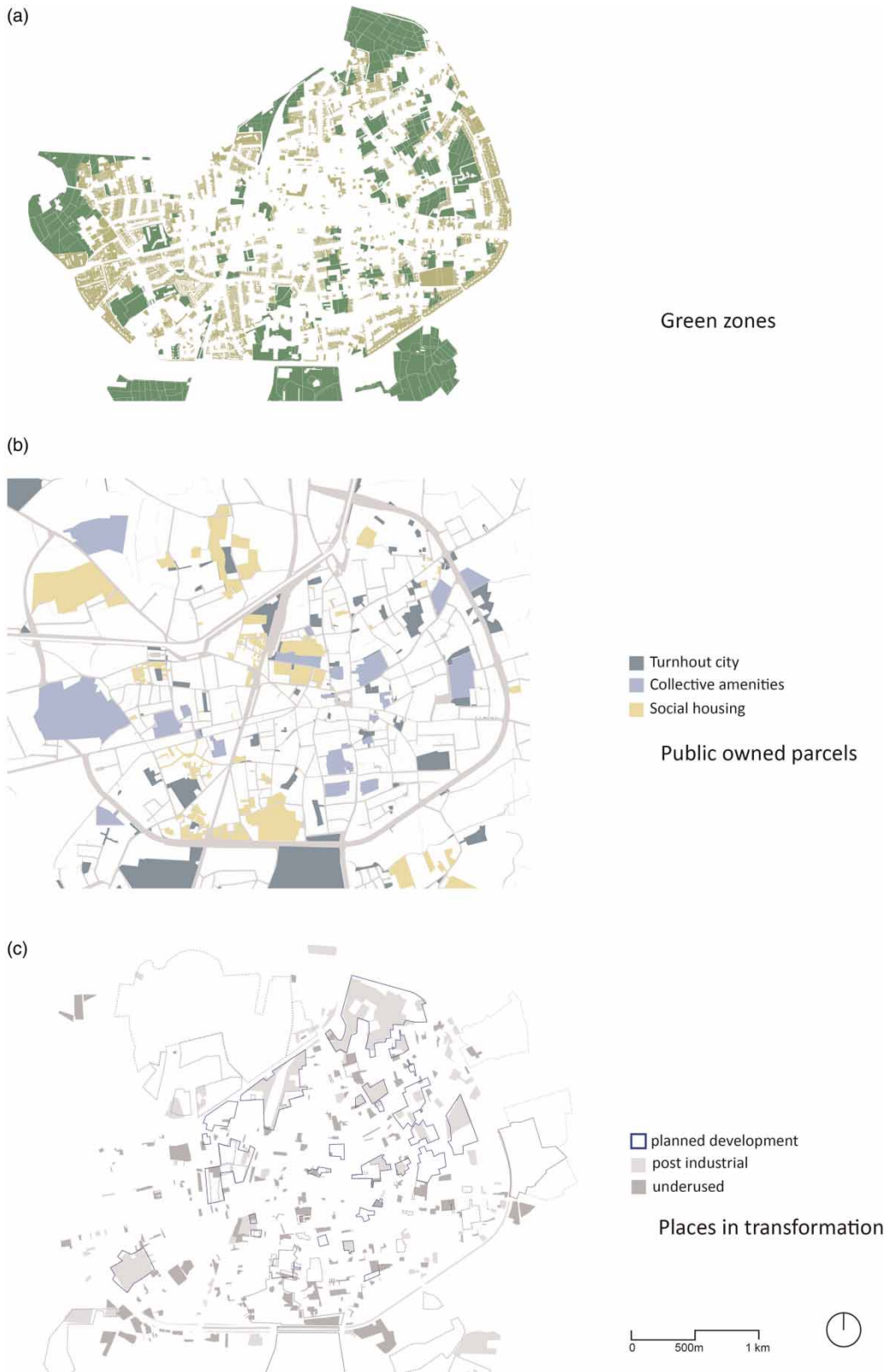
Figure 5 | Identification of the open, green areas for green-blue water integration (Adaptation Option 1) after overlaying the sewer flood locations (not shown), the green zones (a), the public owned parcels (b), and the places in transformation (c) (after Nolf 2013).
