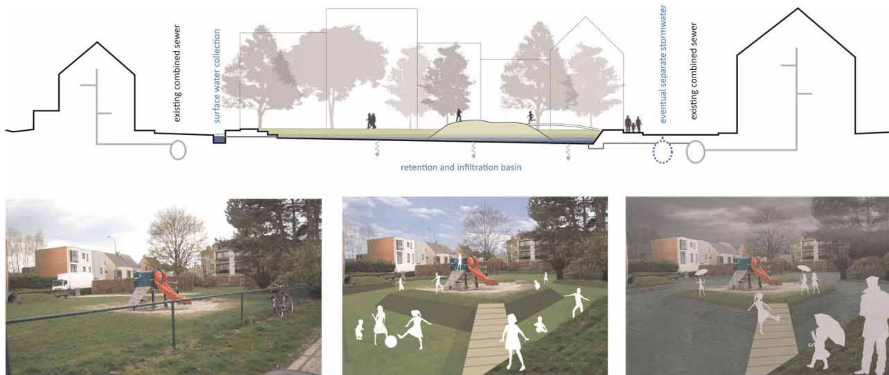
Figure 6 | Example of a designed open, green area for green-blue water integration – converting an existing playground into a multi-use water infiltration/retention facility.
